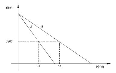
2. **Apply Load Dispenser** on terminal 13 to assign power automatically. The input voltage scope of terminal 13 is 0-9V. When terminal 13 connect with an input 4V, the speed nearly keeps the same as no input connect, so take 4V as a critical value when need to adjust the dispenser. The speed will decrease when the input voltage is increased.
