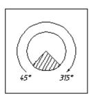
**The SPEED RAMPING Adjustment:** The SPEED RAMPING adjustment is a single coil potentiometer which sets time of adjustment from engine's idle speed to rated speed, the maximum effective adjust angle is 270°. It always points to the mid position when delivered. Rotate the SPEED RAMPING adjustment clockwise to prolong the time(the minimum is 20 seconds), and counterclockwise to shorten it.
