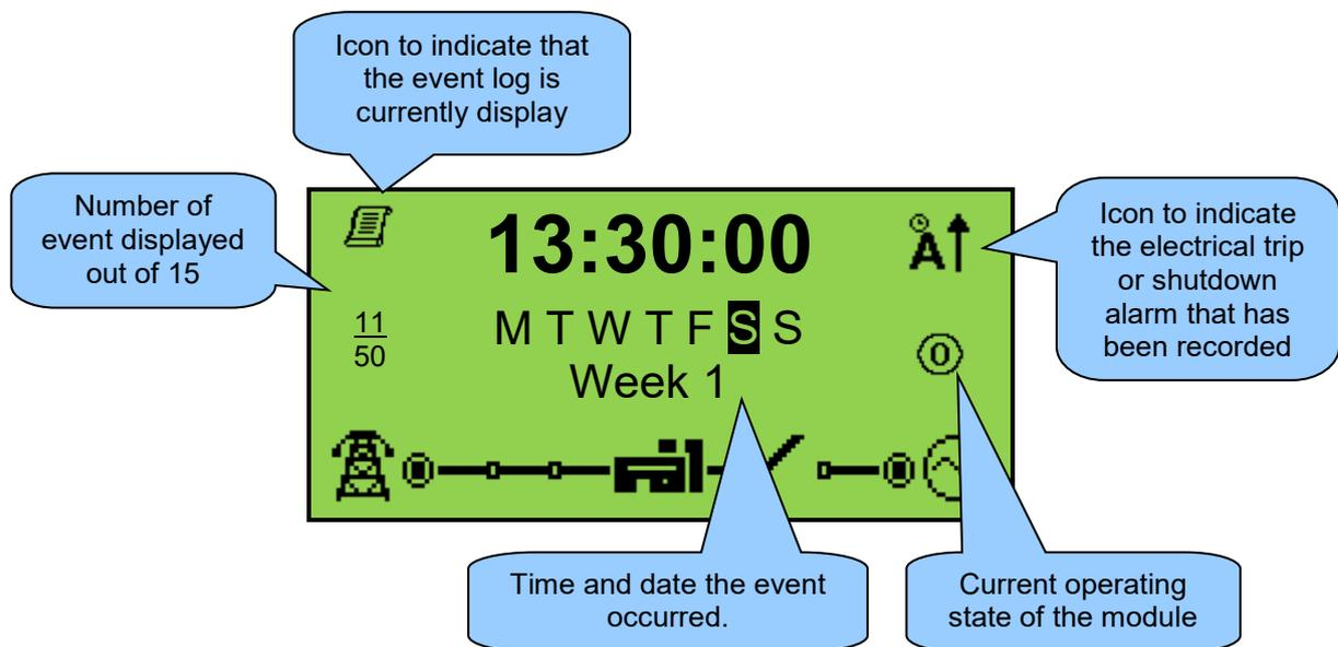
The events shown in the below table are recorded into the module's event log in addition to all electrical trip and shutdown alarms.
