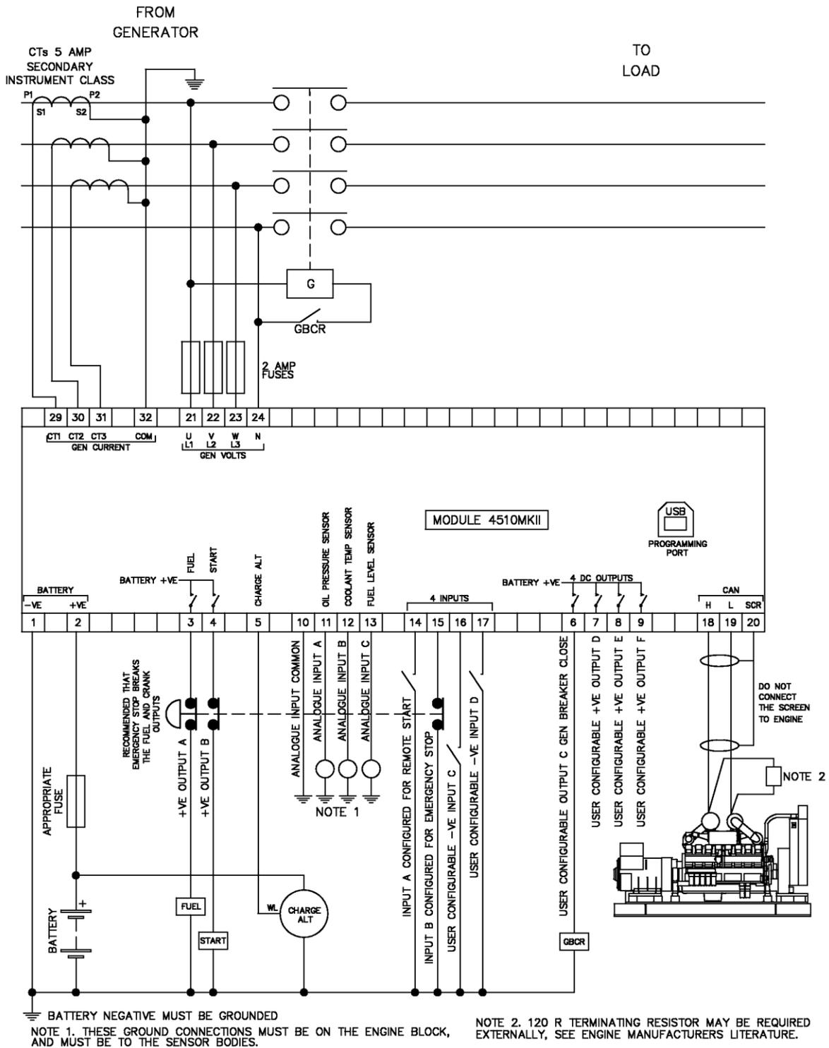
3.3.2 DSE4520 MKII TYPICAL WIRING DIAGRAM (3 PHASE 4 WIRE)
